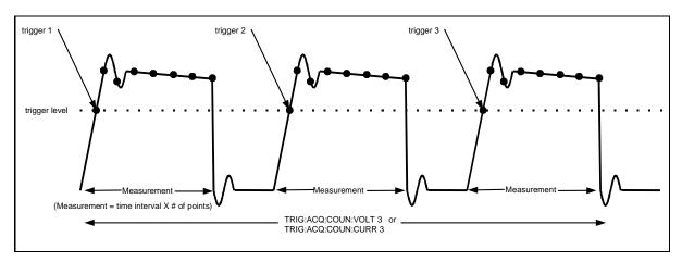
Figure 7-6. Multiple Measurements
